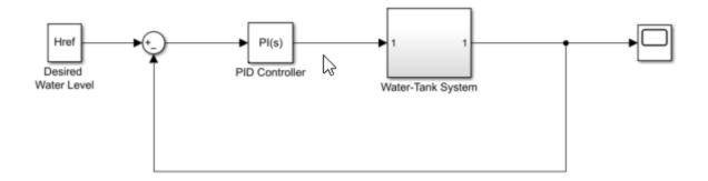
The Water-Tank System block represents the plant in this control system and includes all of the system nonlinearities.
