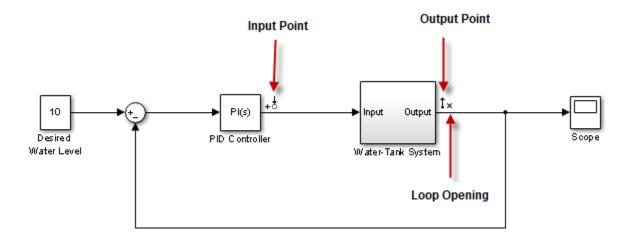
For more information on defining analysis points in a Simulink model, see "Specify Portion of Model to Linearize in Simulink Model". Alternatively, if you do not want to introduce changes to the Simulink model, you can define analysis points using the **Model Linearizer**. For more information, see "Specify Portion of Model to Linearize in Model Linearizer".
